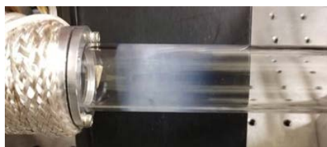
Figure 2: Image of the plasma tube with a white solid deposited on the inner surface due to HAN decomposition.
